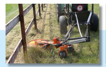
The standard configuration of the SZF/SZL models is a tractor front mount version with hydraulic offset and two support wheels. Cutting width 60 cm.
