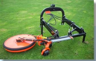
The SZX-850 model has a 85 cm swing arm and is especially designed for attachment to the tractor front lift. The standard configuration includes a hydraulic offset feature, two support wheels and a headstock for front linkage.
