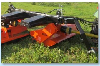
Gearboxes with spiral toothed gears and multiple V-belts assure an indirect flexible drive with maximum security and a minimum maintenance. Two PTO shafts, one wide-angle and one with overrunning clutch deliver an efficient power transmission towards the mower units.
