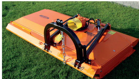
LB-series with hydraulic offset
