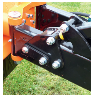
Collision protection in offset arms
